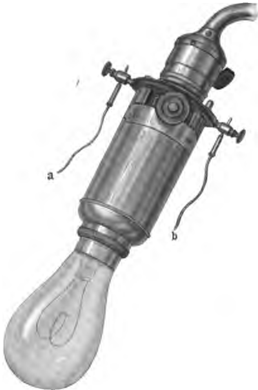
FIG. 147.—A SMALL, VERY CONVENIENT, UNIVERSAL TRANSFORMER OF ELECTRIC CURRENT. It is screwed into the socket of any electric light fixture and transforms any kind of current to one suitable for cystoscope.
